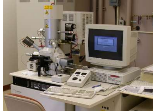
New Focused Ion Beam Milling system (Hitachi FB-2000A) in MTU's "Center for Nanomaterials Research".
